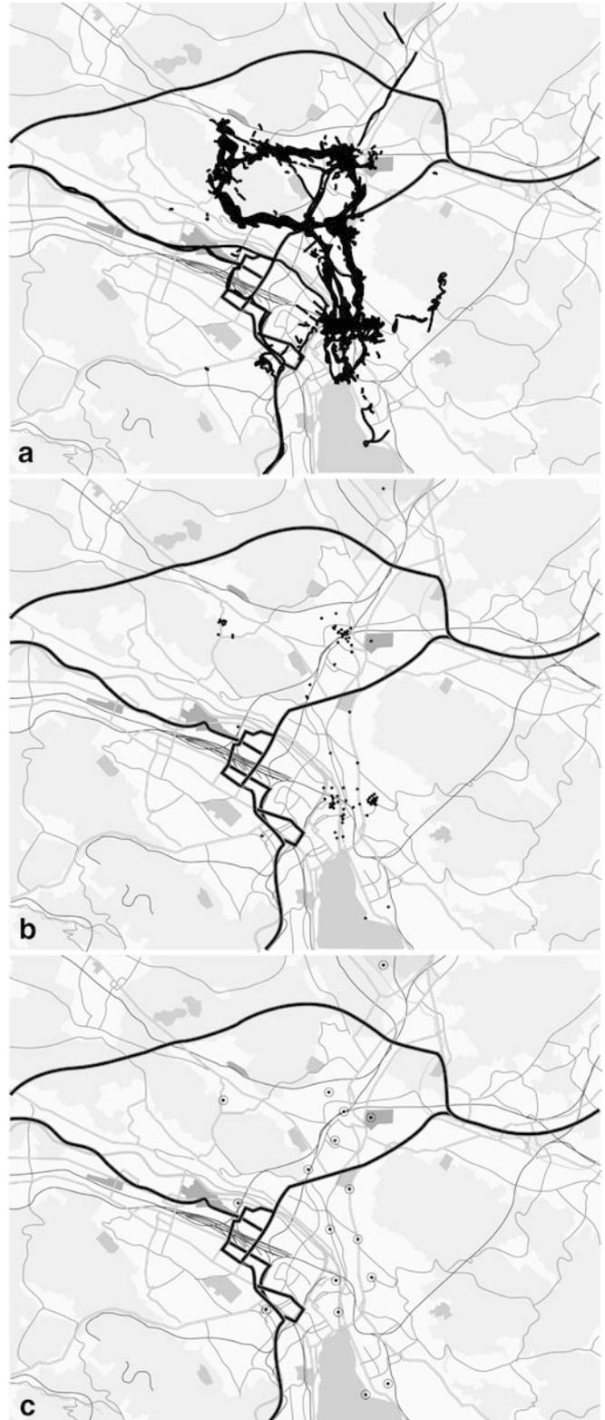
**Fig. 11** An illustration of the data reduction that occurs when creating *places* and *locations*. Picture **a** shows the complete set of data collected in Zürich for one user, around 200,000 data points. Picture **b** shows the roughly 100 *places* that were found using this data. In picture **c**, we see that this has been reduced to just 17 significant *locations*
